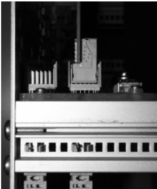
Figure 3. If the depth dimension of the subrack is reduced by 2.5mm, even 13.5mm pins can be used for the hot-swap process.
