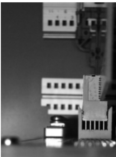
Figure 2. When an 80mm board is pushed into a subrack which conforms to the standard, the connector does not go fully home onto the connecting strip.
