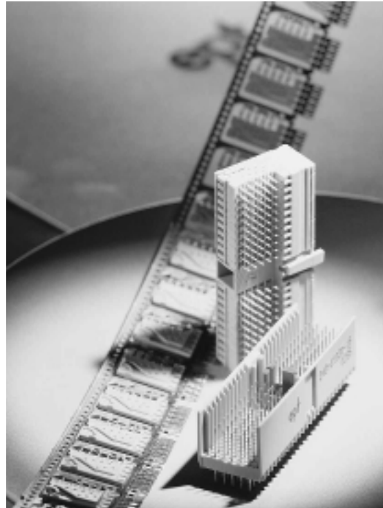
Figure 4. Hard metric connector module A; the guide pins and the coding recess can be clearly seen.
