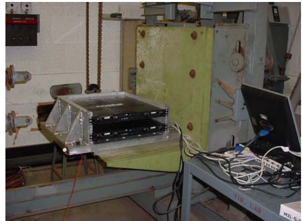
Figure 3, Crystal RS112 in 901D Hammer Blow Testing
