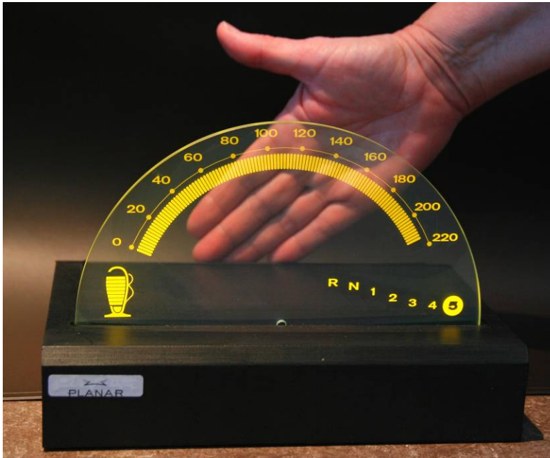
Figure 12 - Transparent EL used in a demonstrator of a heads up display
