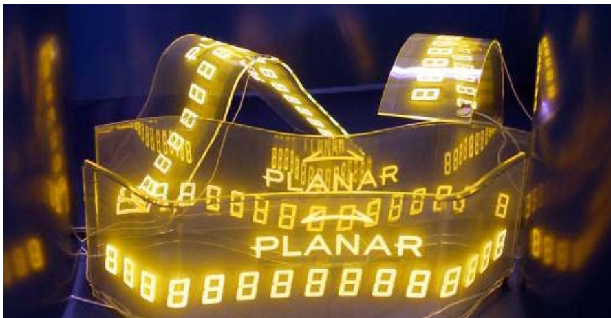
Figure 14 - Demonstration of curved transparent electroluminescent display
